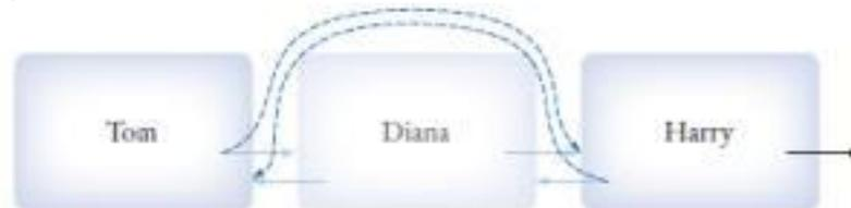
**Figure:** Removing a Node from a Linked List
